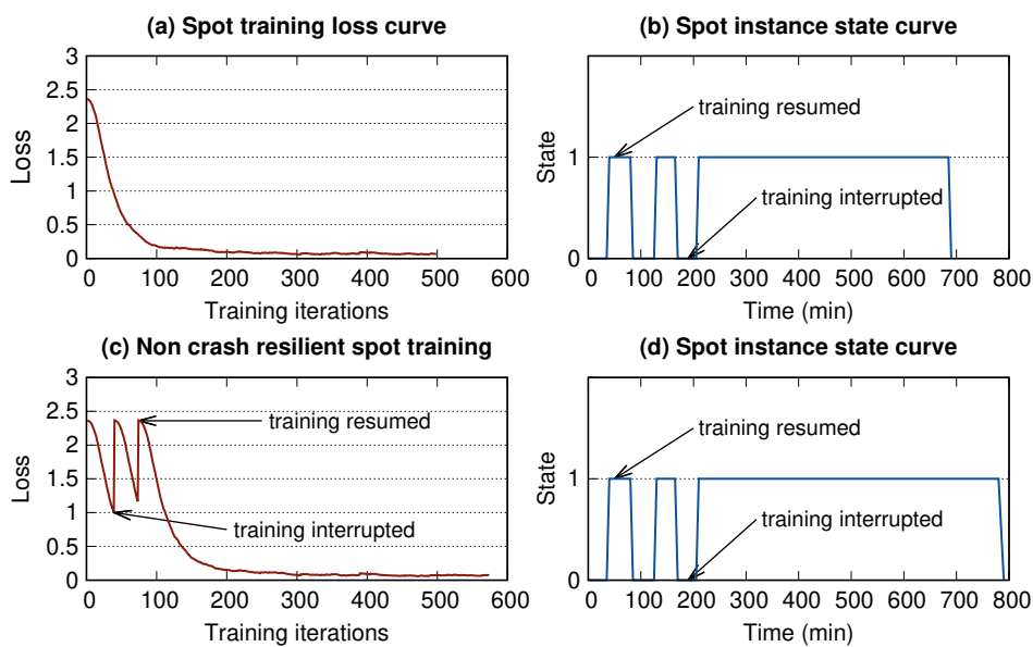
Figure 6.9: Model training with AWS EC2 spot instance traces.
